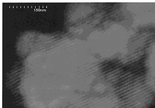
Figure 4. Dark-field TEM image of copper nanowires inside channels of SBA-15.
